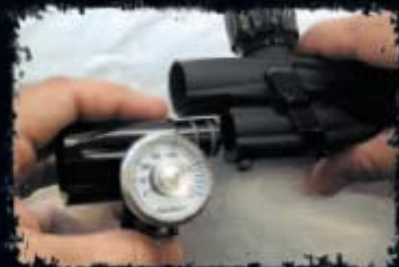
Remove ASA Block From Body
