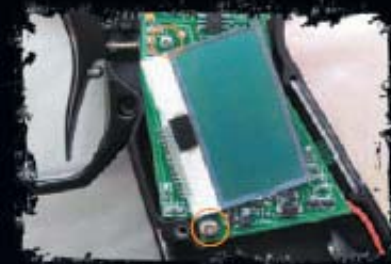
Remove Board Retaining Screws
