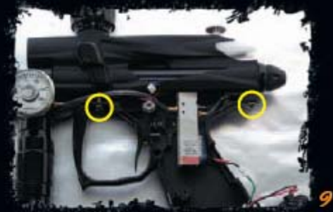
Remove Frame Mounting Screws
