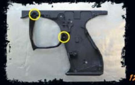
Remove Trigger Guard
