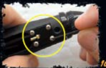
Remove Rear Air Barb Block
