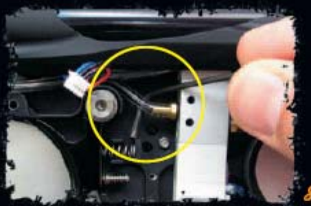
Lift Out Hose From Guard
