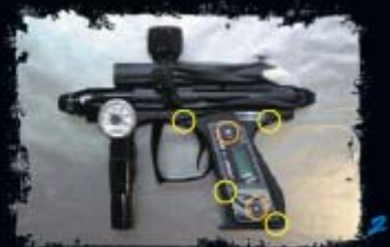
Open Trigger Frame
