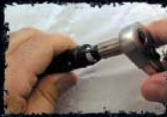
Loosen Valve Using 3/8" Socket
