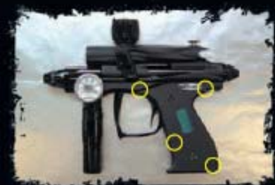
Separate Trigger Halves
