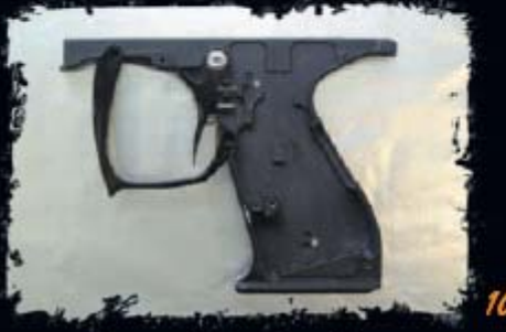
Separate Frame From Body
