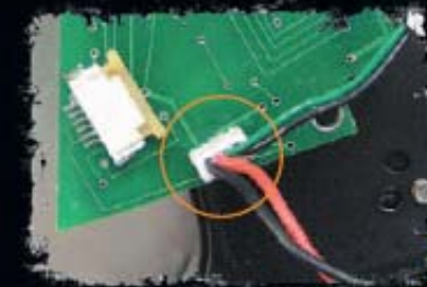
Disconnect Battery Harness
