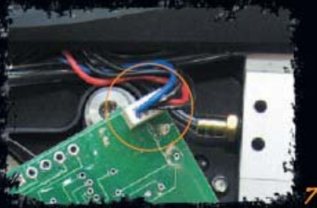
Disconnect Eye Harness, Remove Board
