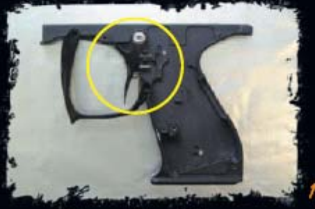
Remove Trigger & Spring
